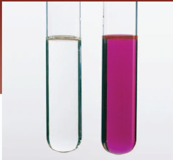
Phenolphthalein in acid and base
