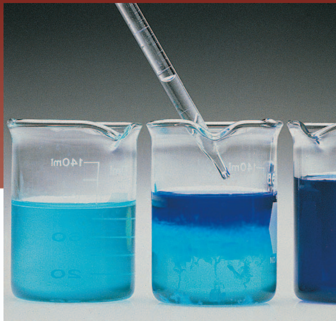
Conversion of \text{Cu}^{2+} to a more complex ion by the addition of ammonia is evidenced by the color change
