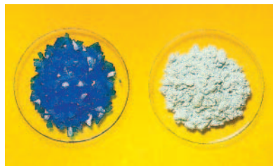
Figure 5.6 Blue Hydrate \text{CuSO}_4 \cdot 5\text{H}_2\text{O} (left), and White, Anhydrous \text{CuSO}_4 (right)
