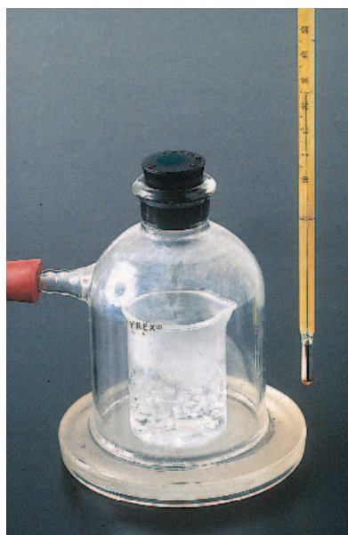
Figure 14.6 Water Boiling at Room Temperature Under Reduced Pressure
